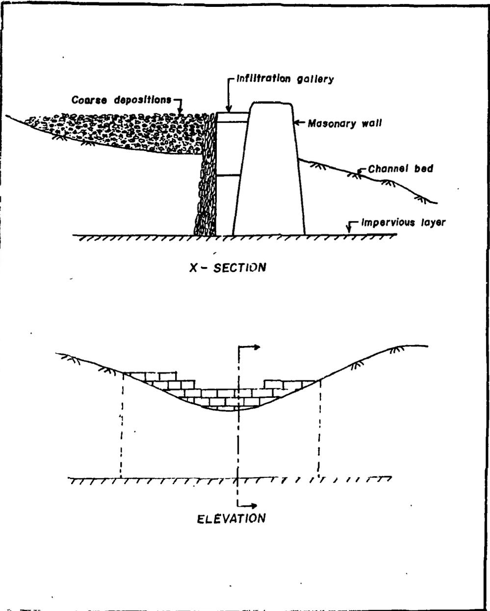
Figure 4 An underground barrage for water harvesting.
