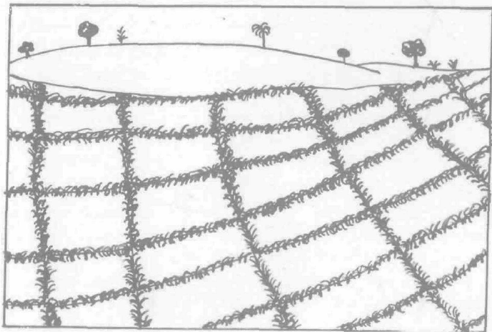
Figure 10 Micro wind breaks for the protection of dune.
