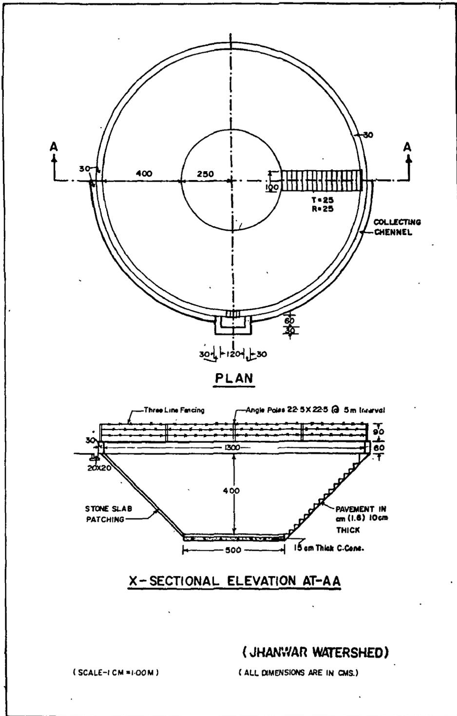
Figure 2 Details of a farm pond of 271 m<sup>3</sup> capacity.
