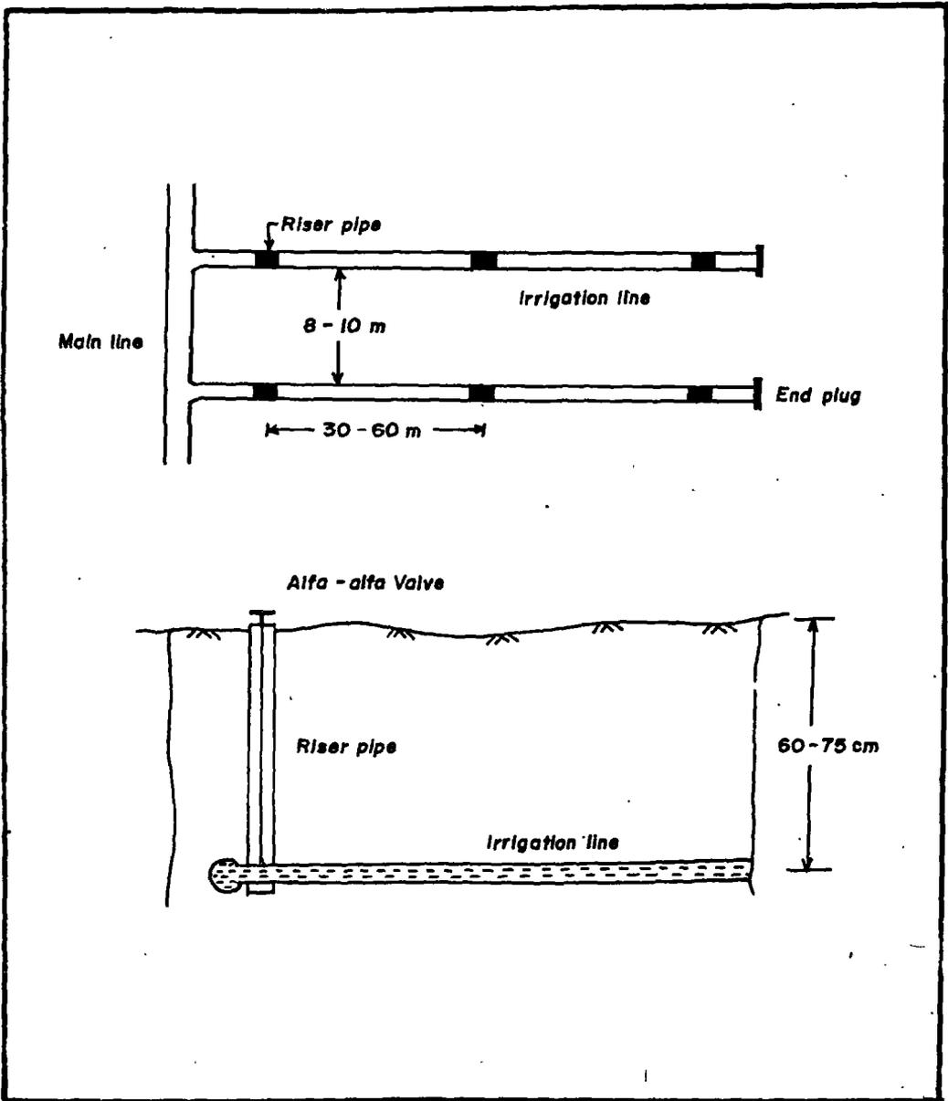
Figure 16 Sub surface irrigation system.
